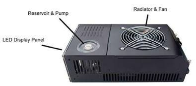
EXT-440 is a compact ambient liquid cooling system. It contains a single 120 mm fan radiator, providing up to 400 W of cooling. Just add coolant, fittings, tubing, and connect to your Andor camera.
