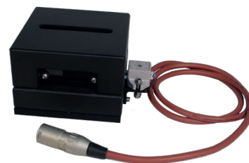
Measuring chamber, electrically heated (C203E)
