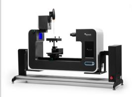
Theta Flow with the Tilting cradle (C204A)
