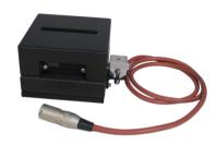
Measuring chamber, electrically heated (C203E)
