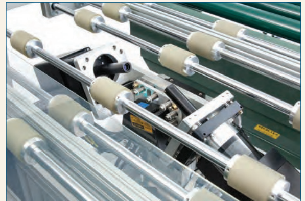
Close-up of In-Line ellipsometer on a conveyor belt.
