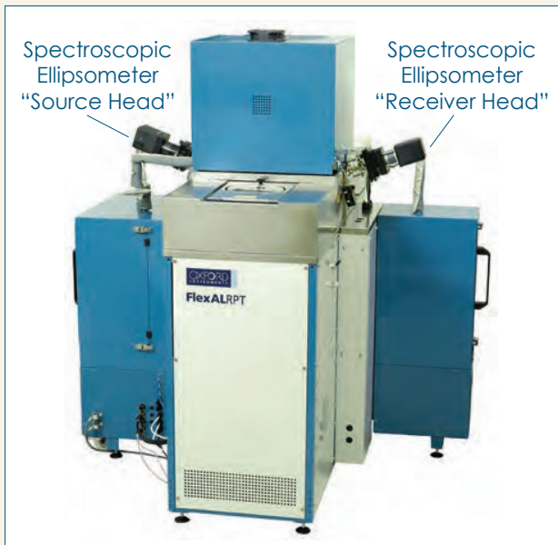
In Situ M-2000 spectroscopic ellipsometer mounted to an Oxford Instruments ALD chamber.
