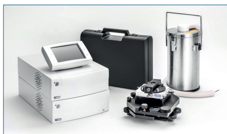
Variable Temperature Stage (-70°C to 600°C)
