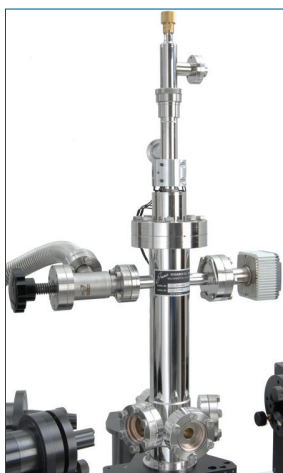
Cryostat (4.2K to 500°C)
