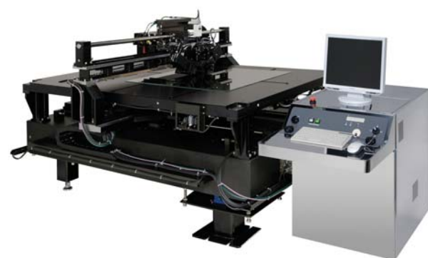
(b) The latest PV mapping tool from Dai Nippon Screen accommodates very large panels. The M-2000 “flies” over the large, stationary panel.
