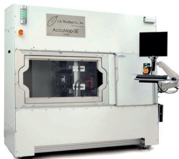
Figure 6. Two large-area mapping tools for PV uniformity measurements. Both incorporate our M-2000 spectroscopic ellipsometer for very fast data at hundreds of wavelengths from the ultraviolet to near infrared. (a) The AccuMap-SE is designed for fast mapping of PV modules up to 1.1 by 1.3 meters.
