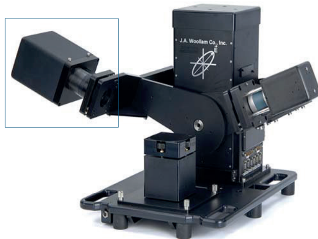
Figure 1. Intensity optimizer on an M-2000 spectroscopic ellipsometer allows convenient control of measurement signal to match the ideal range for any sample.
