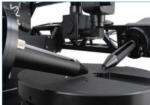
RC2 with automated sample alignment and detachable focusing probes.
