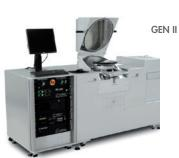
The VUV-VASE variable angle spectroscopic ellipsometer is the gold standard for optical characterization of lithography thin films. It measures wavelengths from vacuum ultraviolet (VUV) to near infrared (NIR). This provides incredible versatility to characterize numerous materials.
