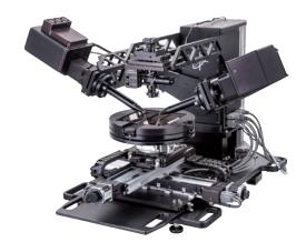
The dual rotating compensator ellipsometers RC2 are new generation of advanced spectroscopic ellipsometry.
