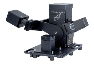
The M-2000 delivers both speed and accuracy. Our patented RCE technology combines Rotating Compensator Ellipsometry with high-speed CCD detection to collect the entire spectrum (hundreds of wavelengths) in a fraction of a second with a wide array of configurations. The M-2000 is the first ellipsometer to truly excel at everything from in-situ monitoring and process control to large-area uniformity mapping and general purpose thin film characterization.
