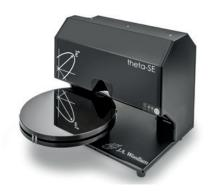
The theta-SE is a push-button spectroscopic ellipsometer for characterizing thin film uniformity. It features advanced ellipsometry instrumentation in a compact package at an affordable price.
