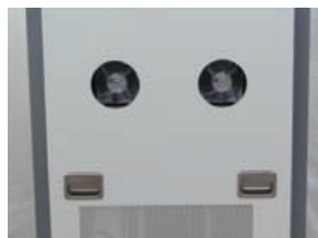
Fans at rear furnace
