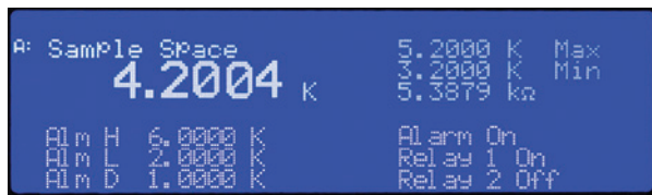
Press any of the 4 input buttons (A, B, C or D) to view or change the parameters for each channel in the input display mode
