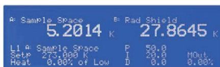
Two input/output display with labels Reading locations can be user configured to meet application needs. Here, the input name is shown above each measurement reading along with the designated input letter.
