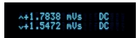
DC positive and negative peak on—the display shows both the positive and negative DC peak readings
