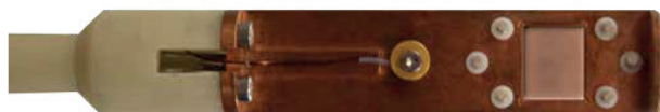
The CCR single sample insert has a sapphire pad and solder posts
