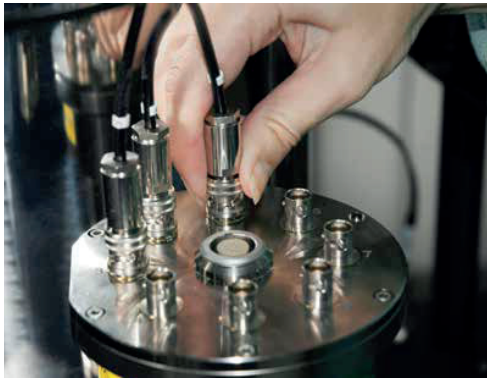
The triaxial cables being attached to the standard insert
