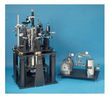
Janis cryogen-free series probe stations provide the researcher with vacuum and cryogenic probing capabilities without requiring the use of liquid cryogens. 4 K, 10 K, and 80 K cryocoolers use proven Gifford-Mc-Mahon (G-M) technology for reliable and affordable sample cooling. Typical applications include MEMS, nanoscale electronics, superconductivity, ferroelectrics, material sciences, and optics.
