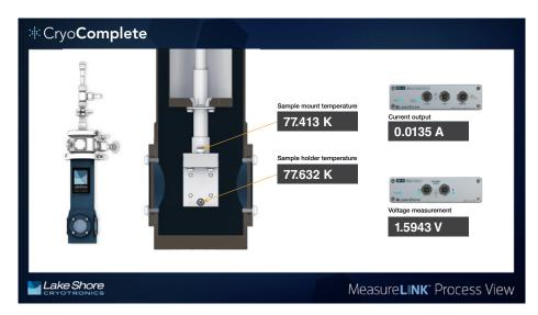
■ Process view shows a representation of the cryostat internals with the appropriate temperatures highlighted for a better understanding of internal temperature variations (shown is an internal view of a VPF-100 application)
