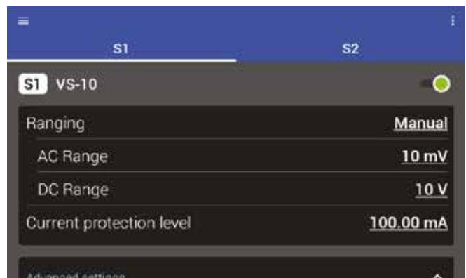
Dual AC and DC range source settings on the VS-10 module enable better control of DC and AC amplitude signals.
