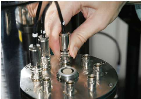
The triaxial cables being attached to the insert
