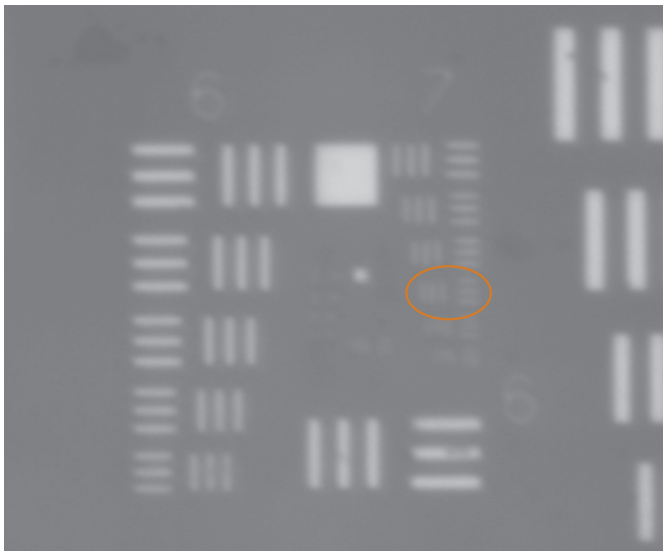
Right: smallest feature visualized (approximately 2.5 µm) obtained with a 12:1 microscope option and coaxial light on a CPX-VF probe station
