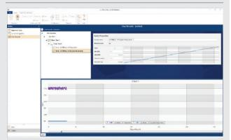
The chart recorder utility enables charting and logging of all system variables, for example, so you can keep a close eye on temperature trends in a cryostat experiment in real-time; it also helps you determine when steady-state conditions have been reached.
