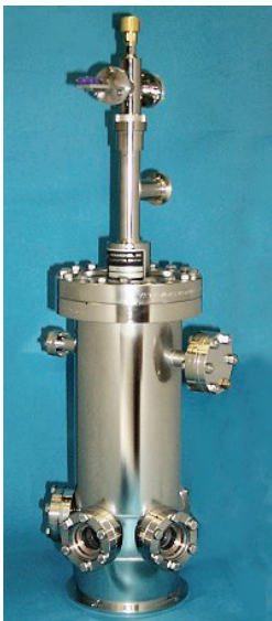
Model ST-400 custom configuration for optical measurements
