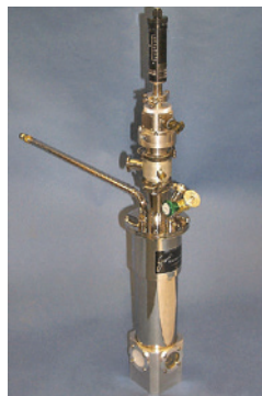
Special STVP-100-2 with manually controlled precision linear manipulator for vertical positioning of samples with 2 in travel, drum dial indicator for vertical axis sample positioner rotation
