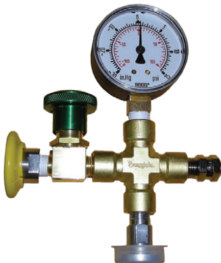
Optional pumping manifold for <77 K operations
