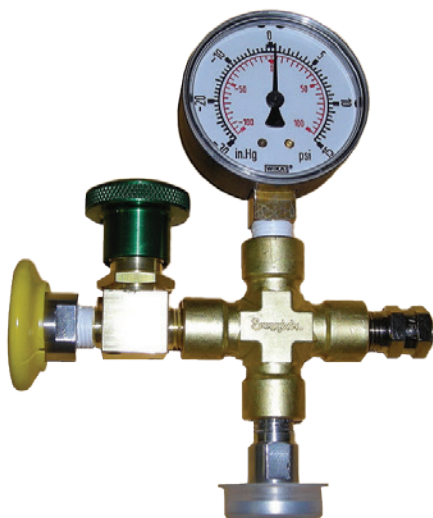
Optional pumping manifold for <77 K operations
