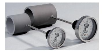
Conical head power probes are used to measure high power density CO<sub>2</sub> laser beams which may damage the standard flat surfaced power probes. The conical absorbing cavity exhibits a high heat dissipation. There are two models of Conical Power Probes: C2K, C4K and C10K. Table 1 below gives specifications for these models. Table 2 gives approximate damage threshold for both the flat surface and conical power probes.
