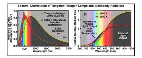
*Figure 1: Tungsten halogen lamp spectrum distribution used for solar simulator*
