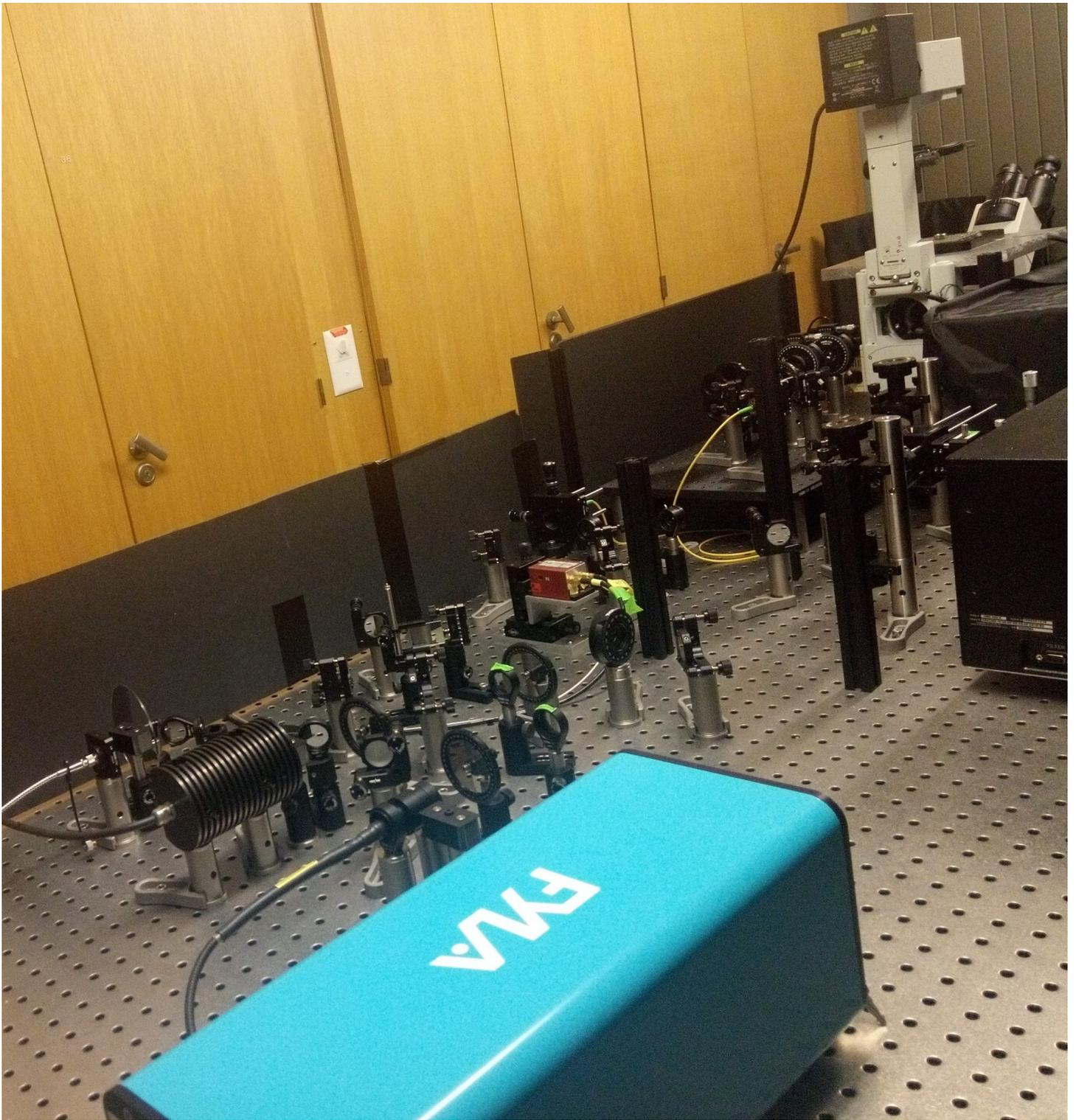
Image of the Photonics Nanosystems Group setup. The fiber-coupled FYLA SCT white laser is guided to the excitation path of a home-built optical confocal microscope. Two additional
