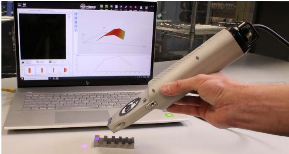
A handheld PSL system measuring a chamfer on an edge break standard.
