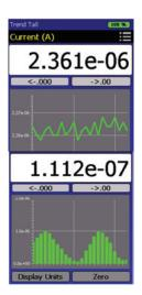
**Trend screen** has all the same features included in meter plus a large easy to read graph showing the readings over time. The graph can be displayed in bar or line graph format. Trend Tall
