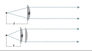
Our condensing optics vary in material and number of lenses, in their spherical aberration and the radiant flux present at the output. The light gathering capability is described by the F/number. As a first approximation the F/number of a lens is given by the ratio of focal length to diameter. The rule of thumb is: the smaller the F/number, the more light can be collected and collimated by a condenser.
