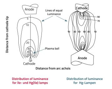
For most applications (especially in spectroscopy) the luminance or radiance is important. As shown in the figure above, Xe arc lamps have one "hot spot" at the cathode while Hg arc lamps have "hot spots" at both electrodes. These plasma balls may be imaged onto pinholes, fibers, monochromator slits or other small targets for maximum illumination (only the plasma ball, not the total area).
