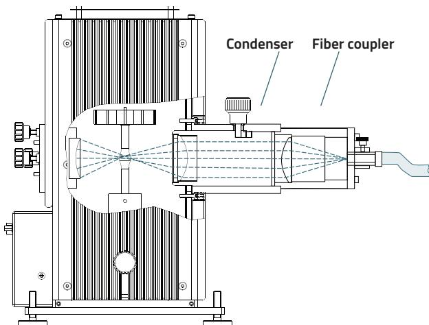
Operation principle of light source with coupled fiber
