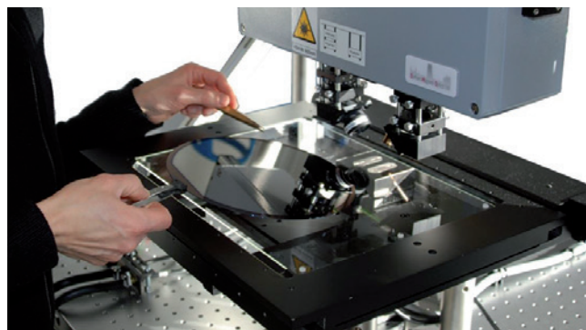
Loading a 200 mm wafer into the NanoMOKE3 Wafer Mapper
