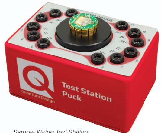
Sample Wiring Test Station
