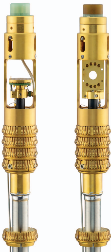
Helium-3 Refrigerator is available either with a horizontal sample stage (left) or a vertical sample stage (right)
