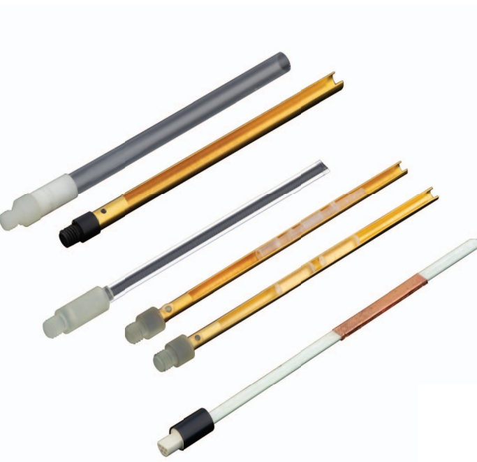
Various sample holders for VSM measurements. The straw holder (top) and large brass trough are only compatible with the LBC, whereas the quartz paddle, small brass trough (with polycarbonate powder holders and quartz bracers shown), and heater stick (for VSM Oven measurements) can all be used with the standard bore coil set.
