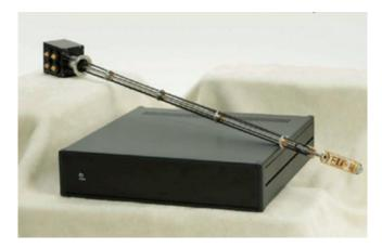
Quantum Design introduces PPMS Ultrasonic option developed as co-development work with Iwate University Japan. The Ultrasonic option can measure elastic constant through special sample probe using ultrasonic sound.
