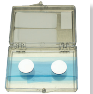
Figure 6: Low tack tape boxes are used for individual or a few small parts.
