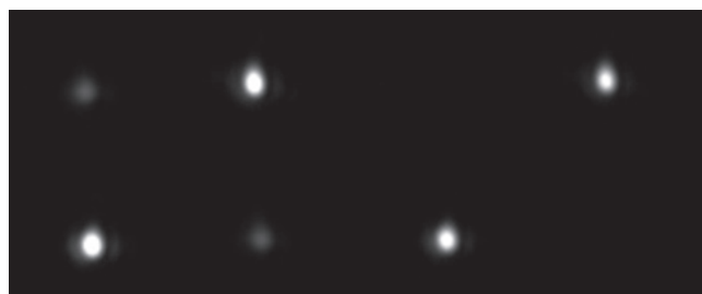
Fig. 7 Ghost traps in conventional time shared tweezer setup (left) and in the Tweez250 system (right)
