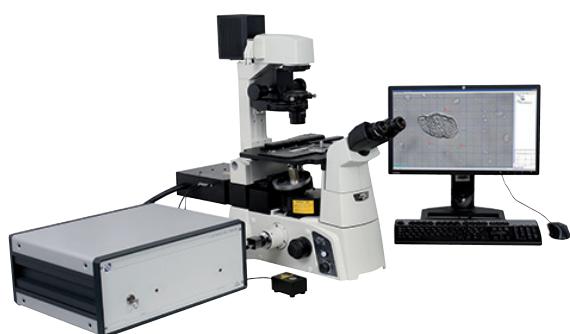
Fig. 1 Aresis Tweez250 optical tweezer mounted on Nikon Eclipse inverted microscope.
