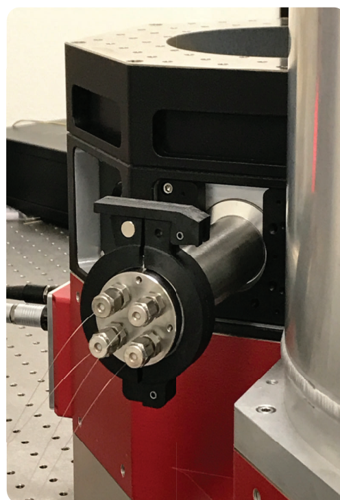
Fiber feedthrough installed in location of one side window.
