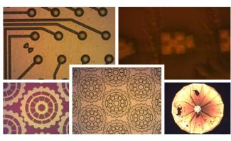
Optical Microscope images of patterns produced across varied types of substrates: Top left: AIN ceramic. Top right: Liquid polymer. Bottom left: Si/SiO<sub>2</sub>. Bottom middle: Glass.
