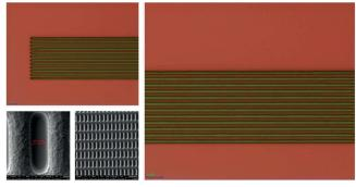
Images of resolutionlimited structures. Top left and right: Lines array with width of 1.0µm and period of 2.0µm on Si/Bottom antireflection coating/S1805 (0.5 µm). Bottom left: Lines array with width of 0.6µm on Si/LOR/S1805 (0.5µm).
