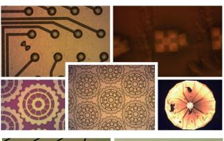
Optical Microscope images of patterns produced across varied types of substrates: Top left: AIN ceramic. Top right: Liquid polymer.
