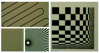
Optical Microscope images of patterns produced on a photomask.
