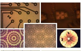
Optical Microscope images of patterns produced across varied types of substrates: Top left: AIN ceramic. Top right: Liquid polymer. Bottom left: Si/SiO<sub>2</sub>. Bottom middle: Glass. Bottom right: Diamond.
