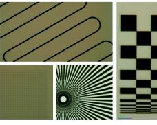
Optical Microscope images of patterns produced on a photomask.
