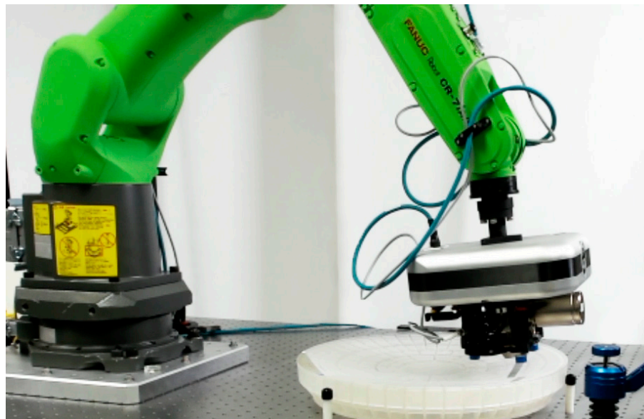
NanoCam HD mounted on robot for production roughness measurements.
