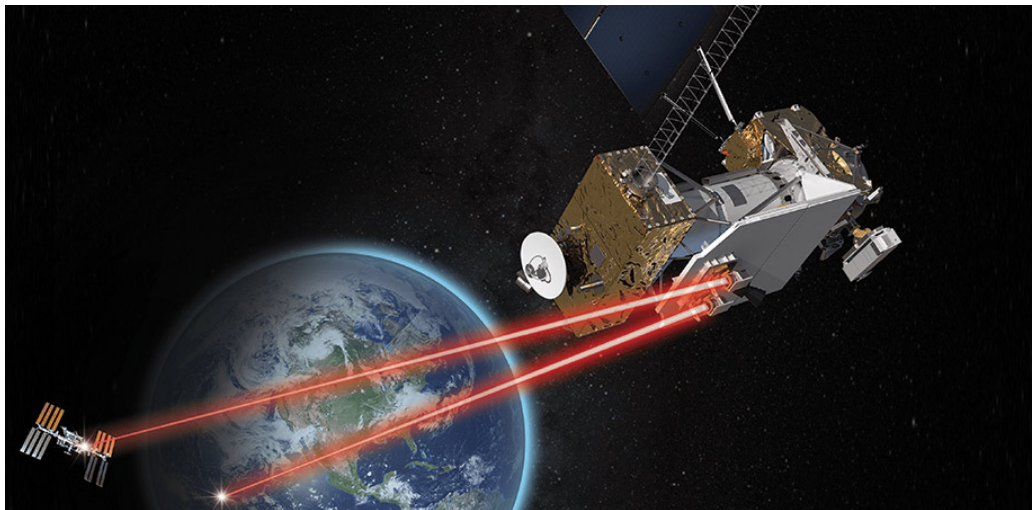
NASA's Laser Communications Relay Demonstration communicating with the International Space Station over laser links. Credit: NASA's Goddard Space Flight Center.
