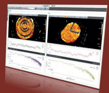
ZYGO's Mx<sup>™</sup> software platform provides full control of the instrument, data acquisition, and analysis. The intuitive interface provides simple navigation and access to 100s of reportable parameters. Advanced analysis tools such as Zernikes, PSD, Corner Cube, Diffraction, PVr, Slopes, and many more are all standard, along with flexible features like scripting and remote access for integrating an interferometer into a larger test setup.
